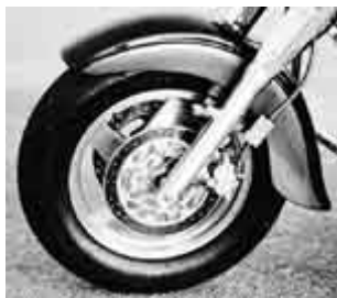
Cast wheels, tubeless tires, dual discs, a stiffer chassis, and revised steering geometry all contributed to the Nomad's success as a tourer.
